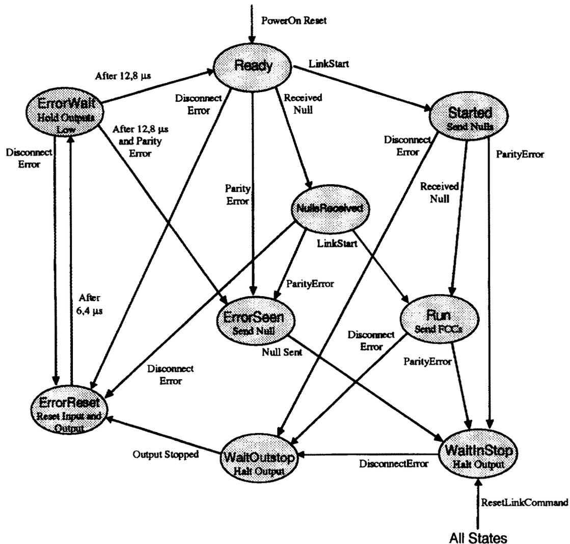
NOTE—In the ErrorReset state, all transitions on the link input shall be ignored, and the flow-control credit counters and input buffer shall be reset.
