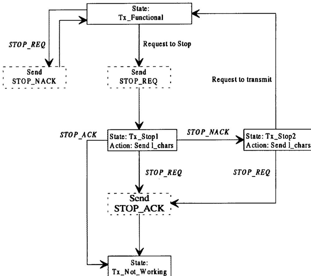
Figure 7-9 —Transmitter state machine controller—shutdown
