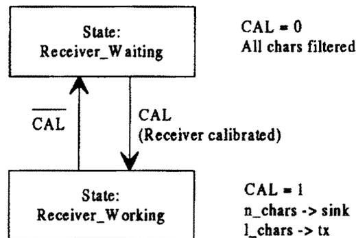
**Figure 7-10 —Receiver state machine controller**
