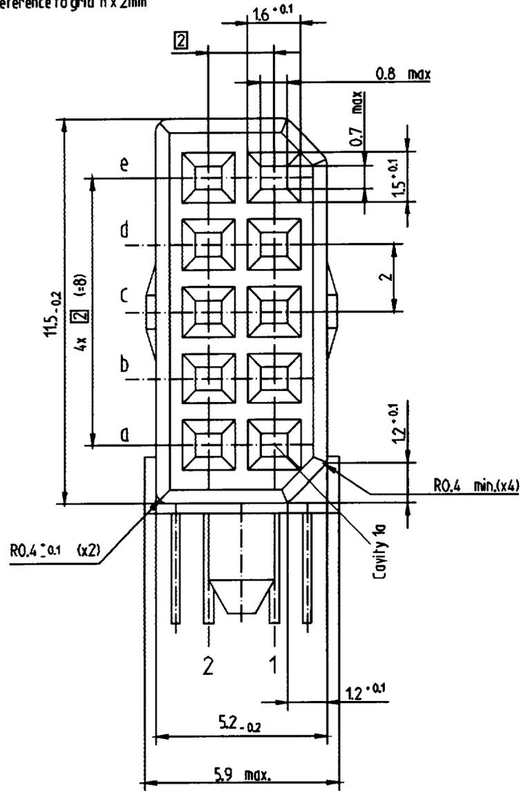
Figure A.1 —DS-DE fixed connector front view
