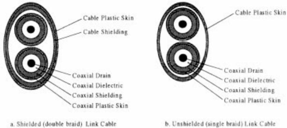
**Figure 7-1 —Single braid and double braid link cables**
