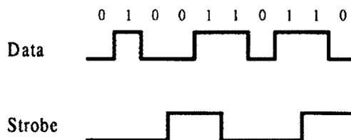
**Figure 5-4 —DS-SE link signal encoding**
