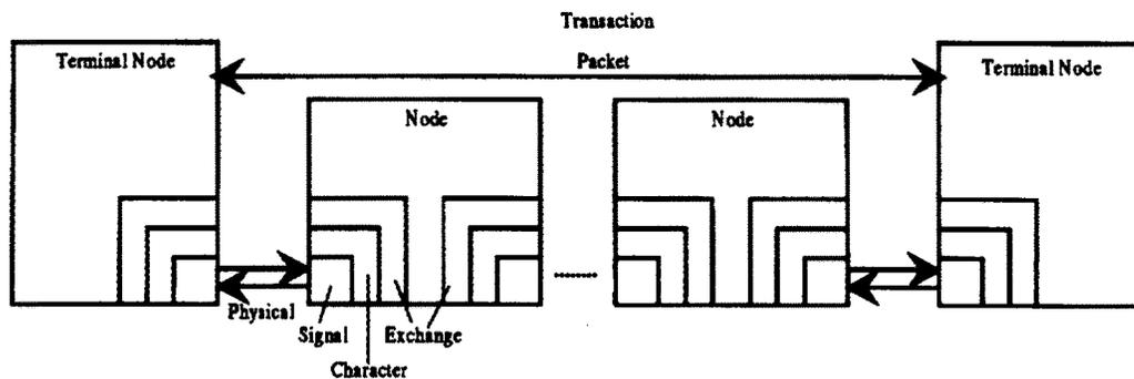
Figure 4-1 —Protocol stack between nodes
