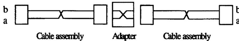
**Figure 7-3 —HS-SE extension adapter**
