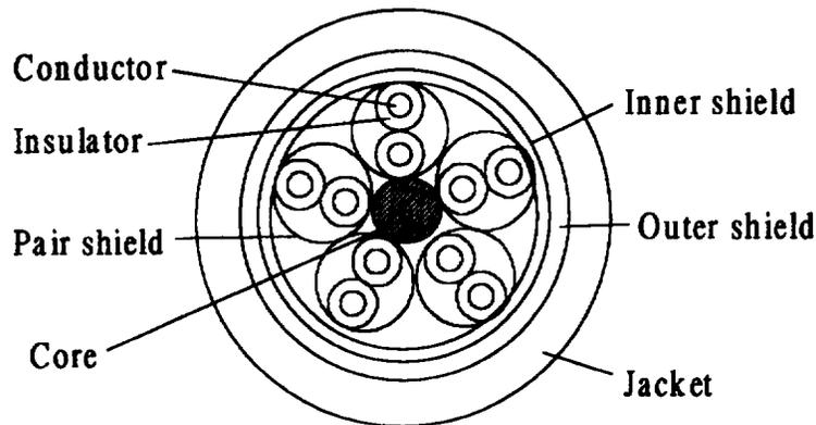
Figure M.1—Recommended DS-DE link cable cross section
