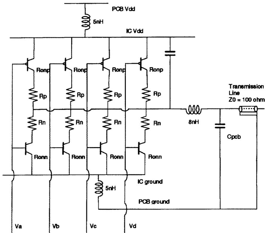
Figure J.1—S-SE pad equivalent circuit
