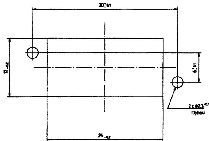
Figure N.2—DS-DE (multiway) front panel cut-out
