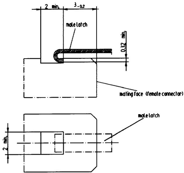
Figure B.5 —HS-SE connector link
