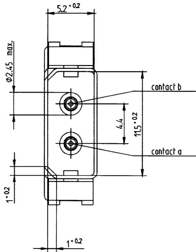
Figure B.1 —HS-SE free connector front view
