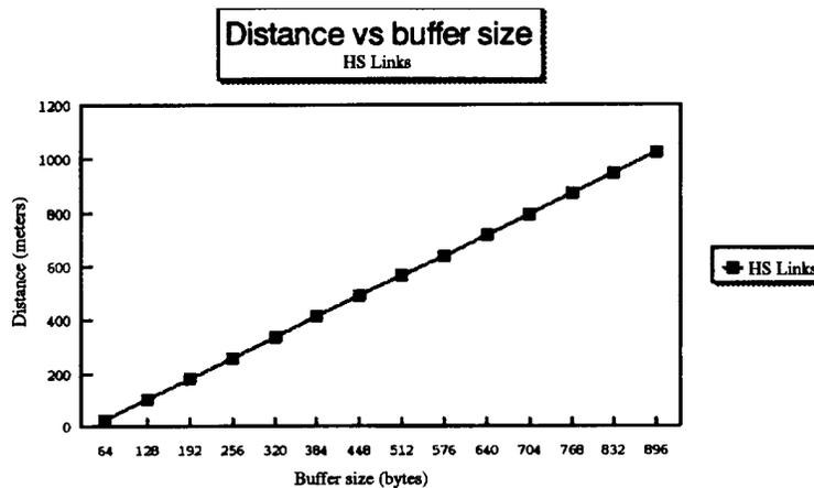
Figure H.3—Distance vs. buffer size for HS-SE links
