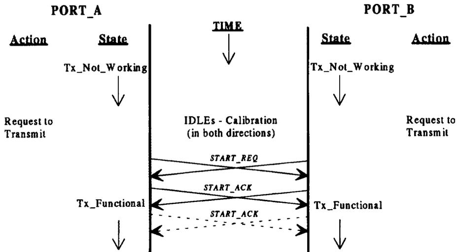
Figure 7-12 —Exchange for bidirectional start-up
