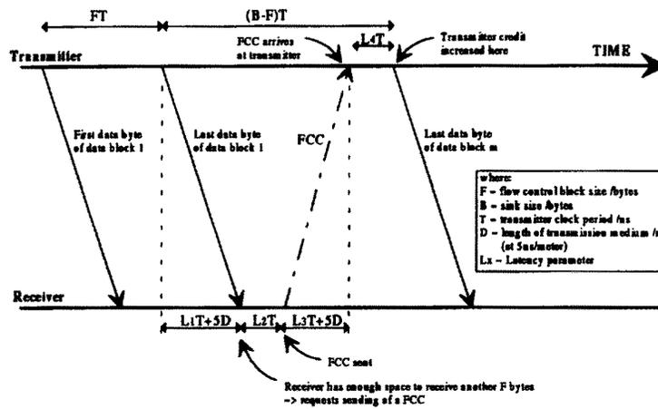
Figure H.1—Theoretical maximum transmission length calculation
