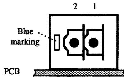
Figure 6-3 —TS-FO fixed adaptor, external view and ferrule allocation
