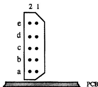
Figure 5-7 —DS-DE fixed connector external view
