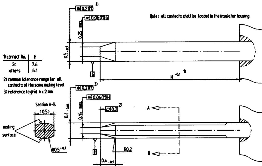
Figure A.7 —DS-DE free connector contact
