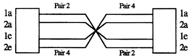
Figure 5-5 —DS-DE cable assembly twist example
