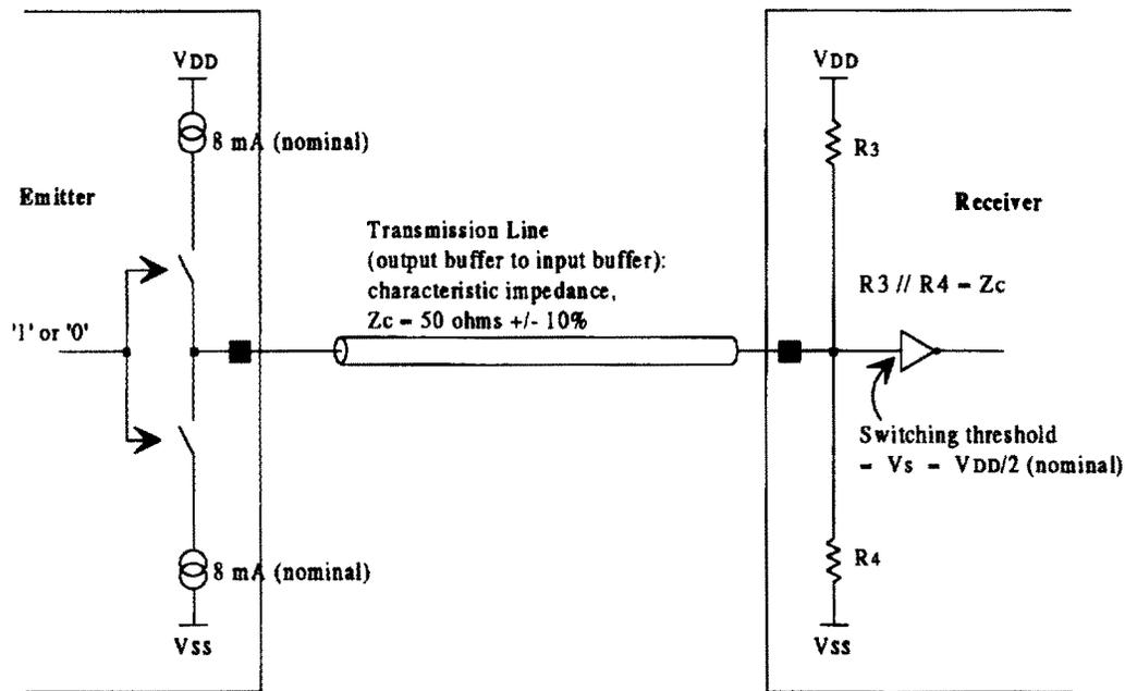
**Figure 7-5 —Input and output buffer electrical model**
