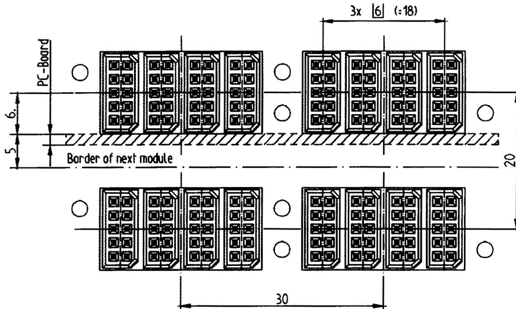
Figure N.1—DS-DE connector multiway housing
