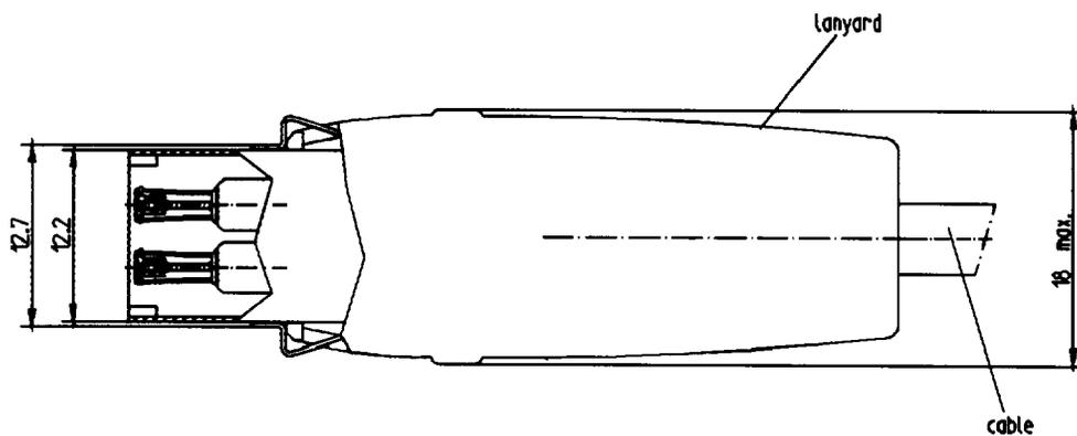
Figure B.2 —HS-SE free connector side view
