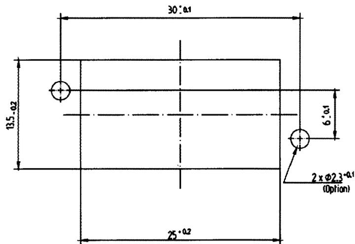
Figure Q.2—HS-SE (multiway) front panel cut out
