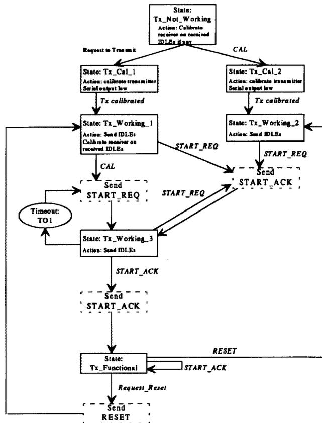
Figure 7-7 —Transmitter state machine controller—start-up
