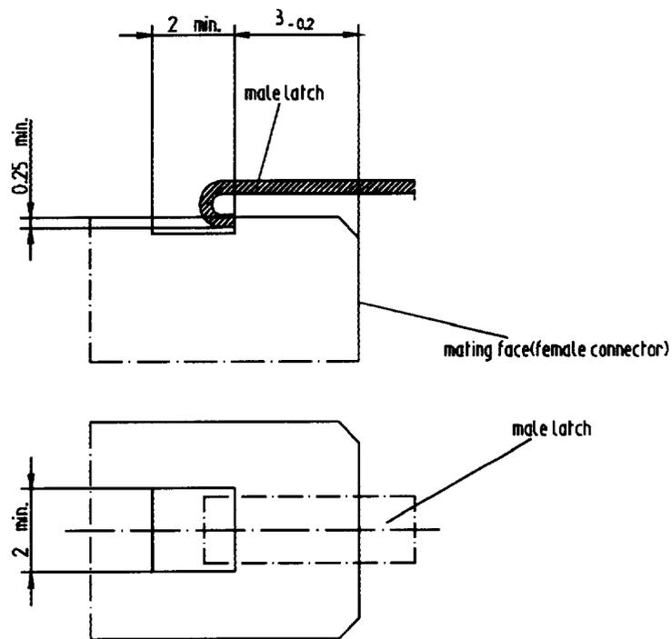
Figure A.4 —DS-DE connector latch
