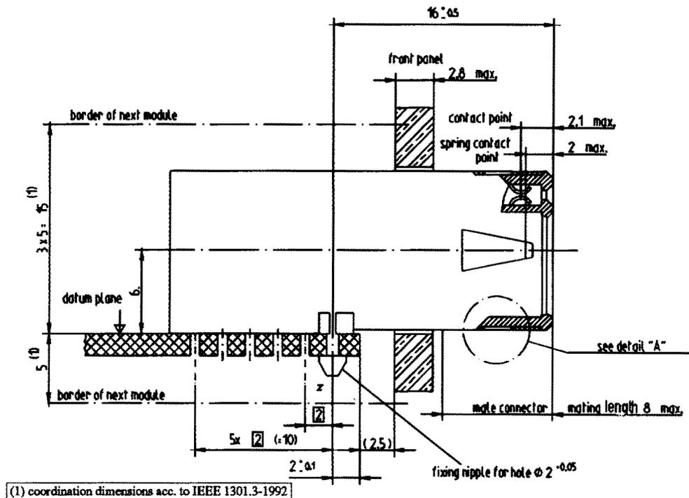
Figure A.2 —DS-DE fixed connector side view
