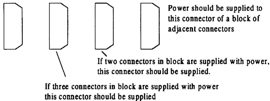
Figure 5-8 —Multiple power connectors
