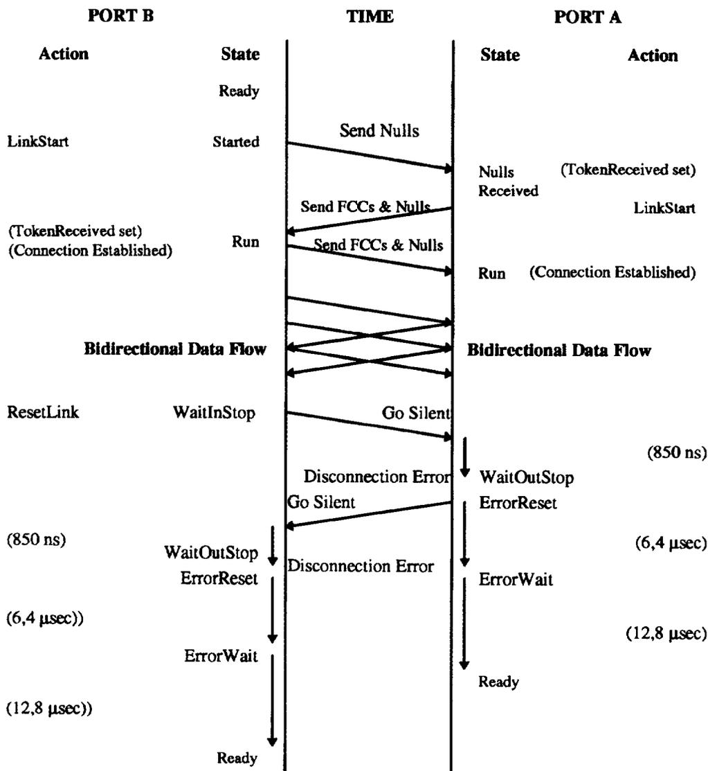
Figure 5-12 —DS link start-up and reset
