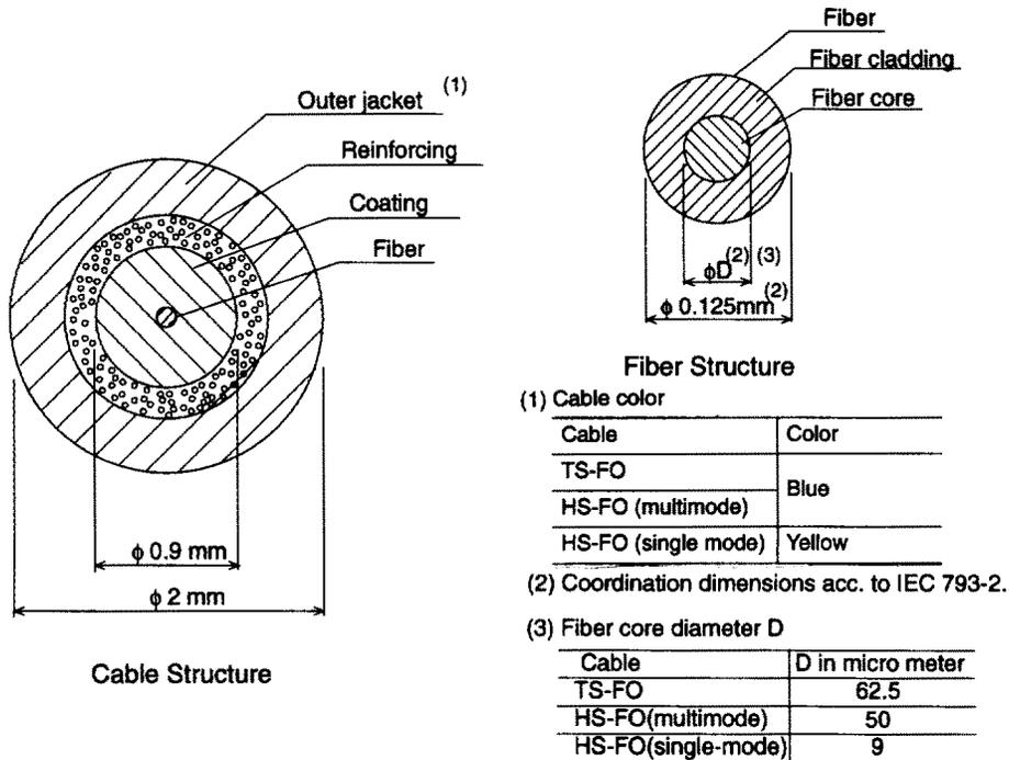
Figure S.1—Example of TS/HS-FO fiber cable structure
