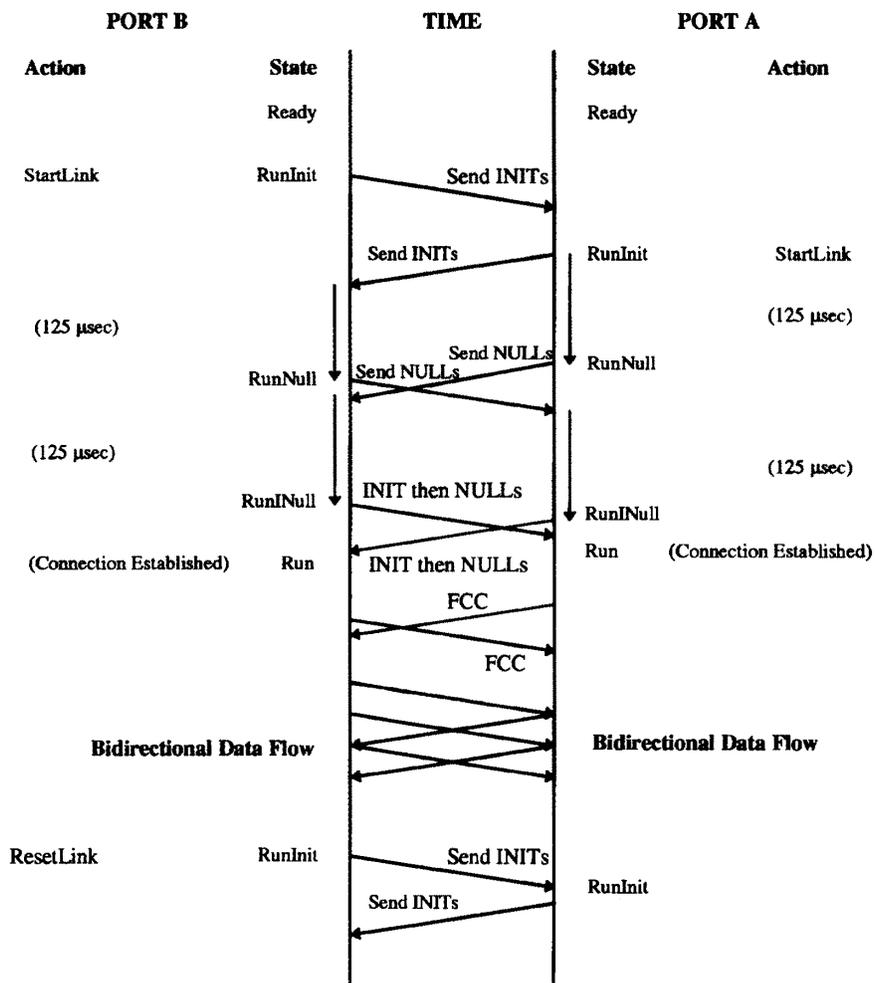
Figure 6-6 —TS link start-up and reset
