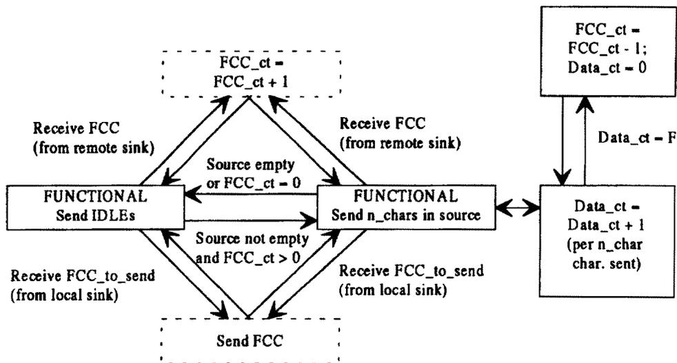
Figure 7-8 —Transmitter state machine controller—functional
