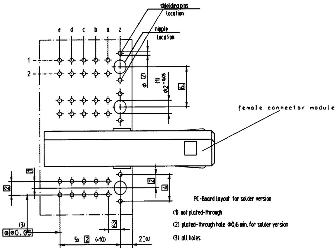
**Figure L.1—DS-DE fixed connector PCB layout**
