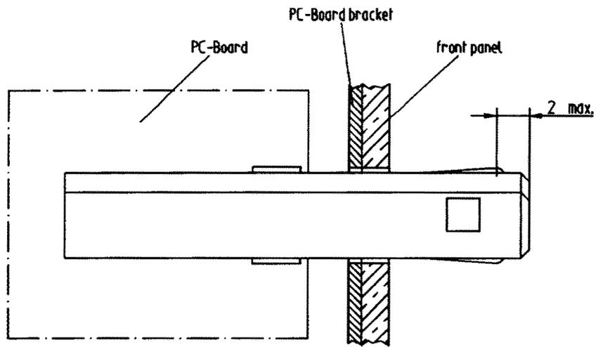
Figure A.3 —DS-DE fixed connector top view
