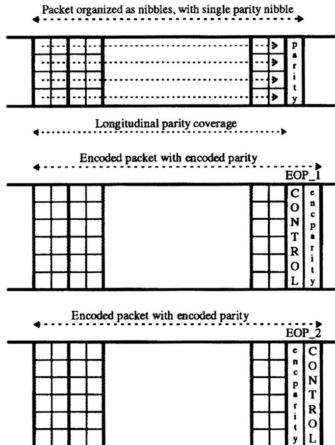
Figure 6-7 —TS-FO packet encoding
