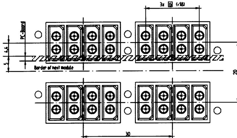
Figure Q.1—HS-SE multiway housing
