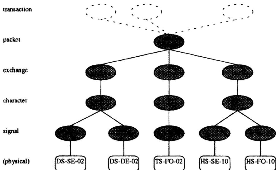
Figure 4-4 —Defined implementations of physical and logical layers
