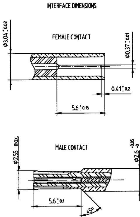
Figure B.6 —HS-SE contact interface dimensions
