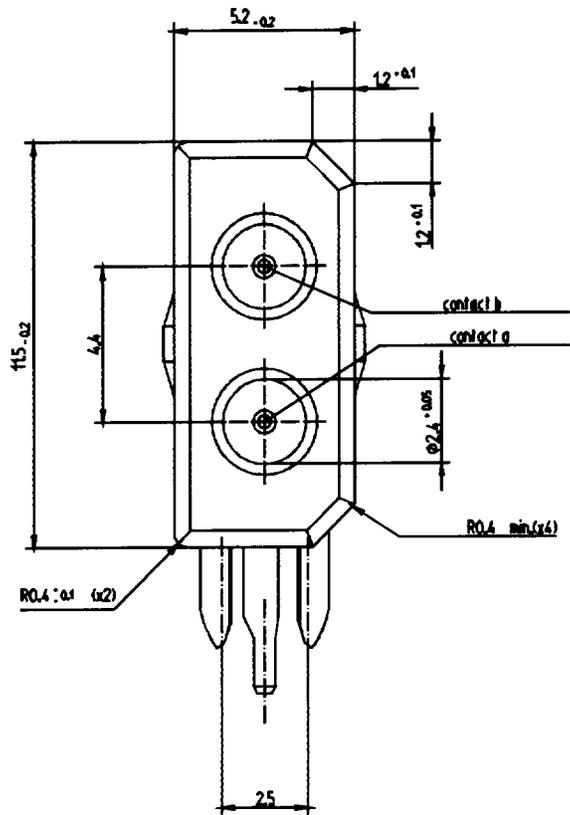
Figure B.3 —HS-SE fixed connector front view
