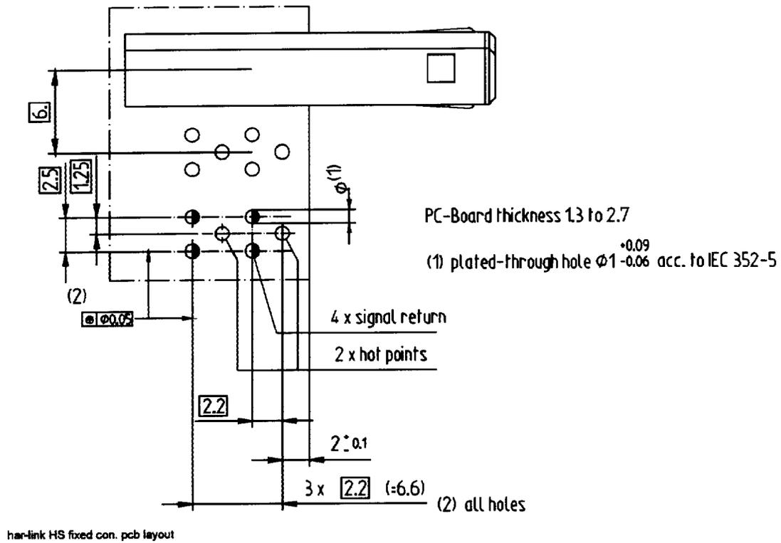
Figure O.1—Recommended HS-SE fixed connector PCB layout
