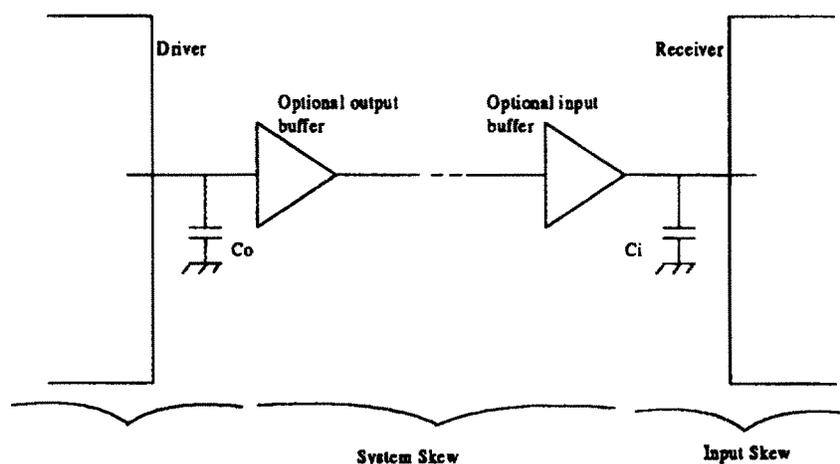
**Figure 5-2 —DS-SE timing reference model**
