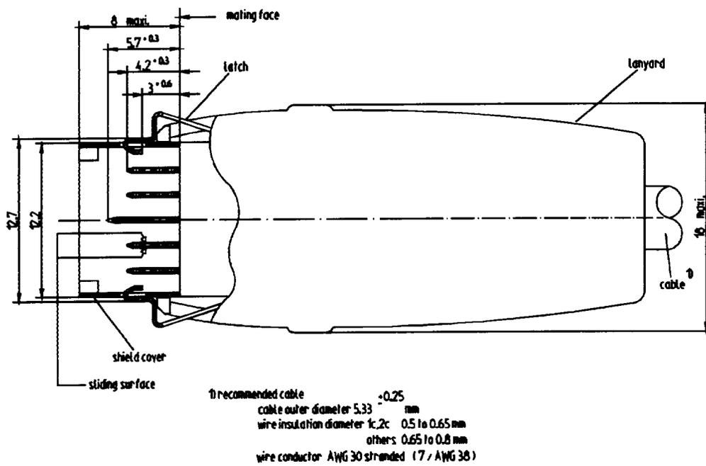
Figure A.6 —DS-DE free connector side view
