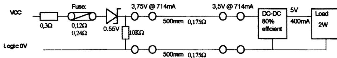
Figure K.1—Optional power supply circuit
