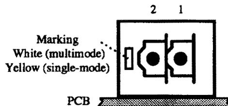
**Figure 8-3 —HS-FO fixed adapter, external view and ferrule allocation**
