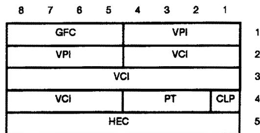
**Figure F.5 —ATM cell header**
