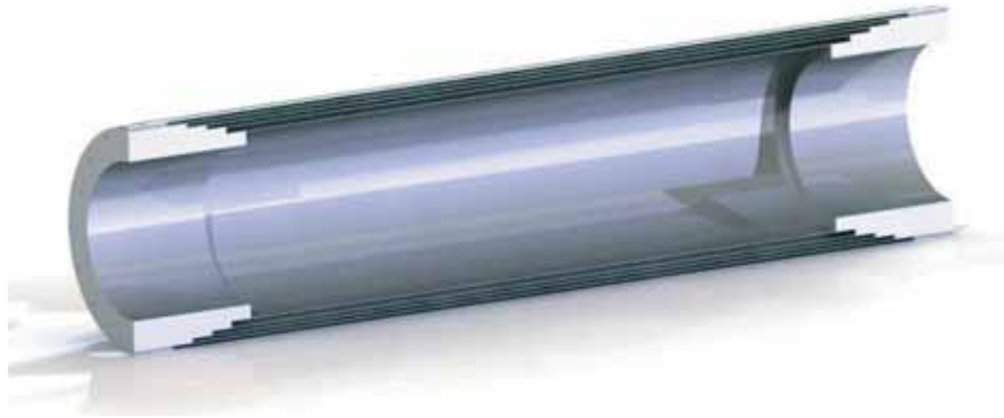
Figure 4: Schematic structure of the cylindrical triple-GEM detector C0
