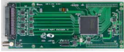
Figure 20: Pipeline TDC FINESSE card base on FPGA
