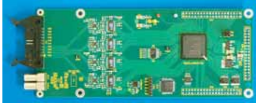
Figure 19: Flash ADC FINESSE card with 65 MHz sampling
